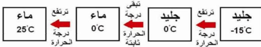
$$\begin{aligned} Q_1 &= m C_{ice} \Delta T \\ &= 2 \times 2093 \times [0 - (-15)] \\ &= 2 \times 2093 \times 15 \\ &= 30 \times 2093 \end{aligned}$$
